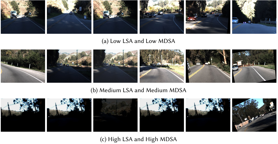
Fig. 3. Synthetic images for Chauffeur model generated by DeepTest. The three images on the left are picked based on LSA and three images on the right are picked based on MDSA. Images with higher LSA or MDSA values tend to be harder to recognise and interpret visually.
